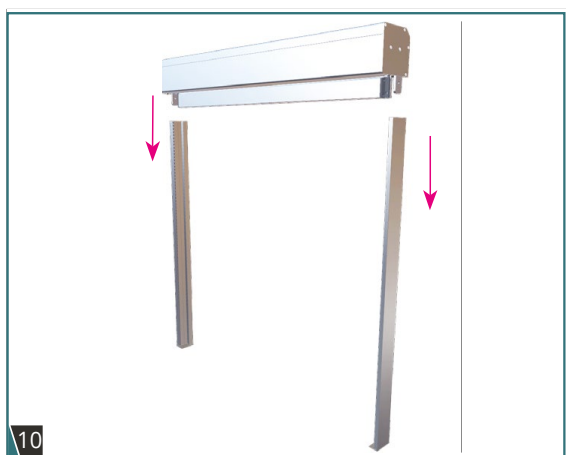
Fig. 10. Apply the cassette to the guides. Correct installation of brackets guides and cassettes: every 70 cm.
