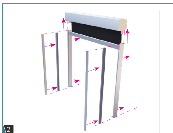
Fig. 2. Check that the system is complete and compatible with order. Measure the cassette and guides.
